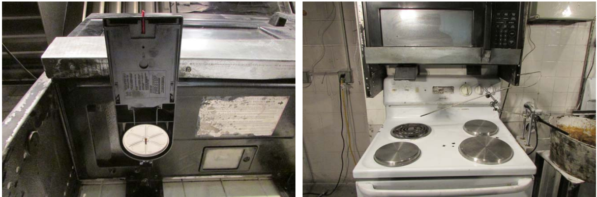
Figure 3. Stovetop Firestop® Installed Prior to a Fire Test.
