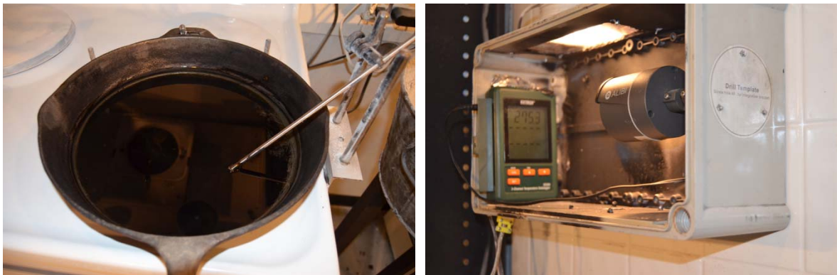
Figure 5. Oil Temperature Measurement (Left: Thermocouple Probe, Right: Data Logger).
